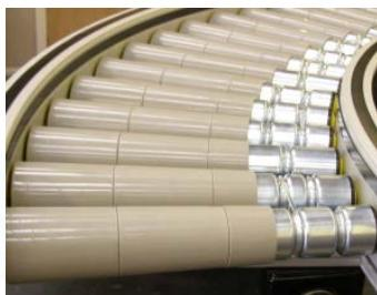
Line shaft roller conveyor is a powered conveyor system. It has the capability of accumulating products with minimum back pressure. Typical characteristics include quiet operation and easy maintenance. Suited for many applications, including: side loading conveying, smooth merges and low pressure accumulation application conveying
