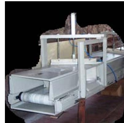
Mitmol Belt Trippers / Plows create multiple discharge points for a belt conveyor. Typically, a belt conveyor can only discharge bulk materials off the end of the belt. Belt Trippers are short belt conveyors that can be positioned at different points along a main belt conveyor to "trip" or divert the flow of bulk materials off through a chute.
